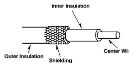
5. Pull the shielding to one side. Connect the center wire to the receiver's **FM UNBAL 75** $\Omega$  terminal. Twist the shielding to secure any loose wire strands, and connect it to the **GND** terminal.
